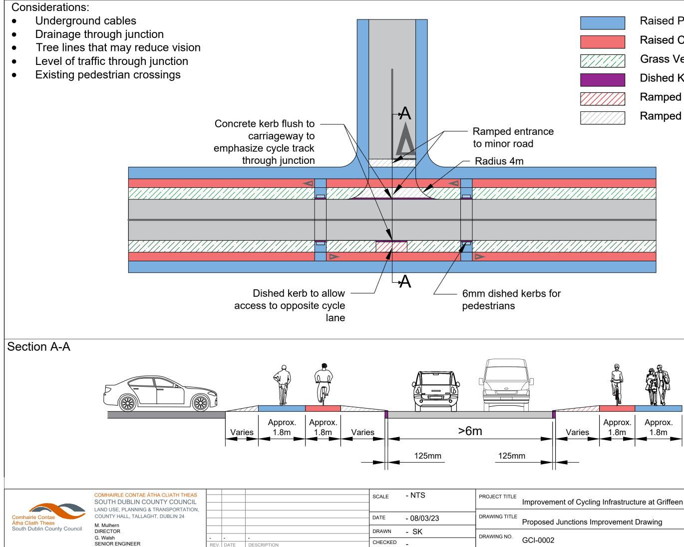
Raised Pedestrian walkway Raised Cycle Track **Grass Verge Dished Kerb** Ramped Cycle Track Ramped Road
