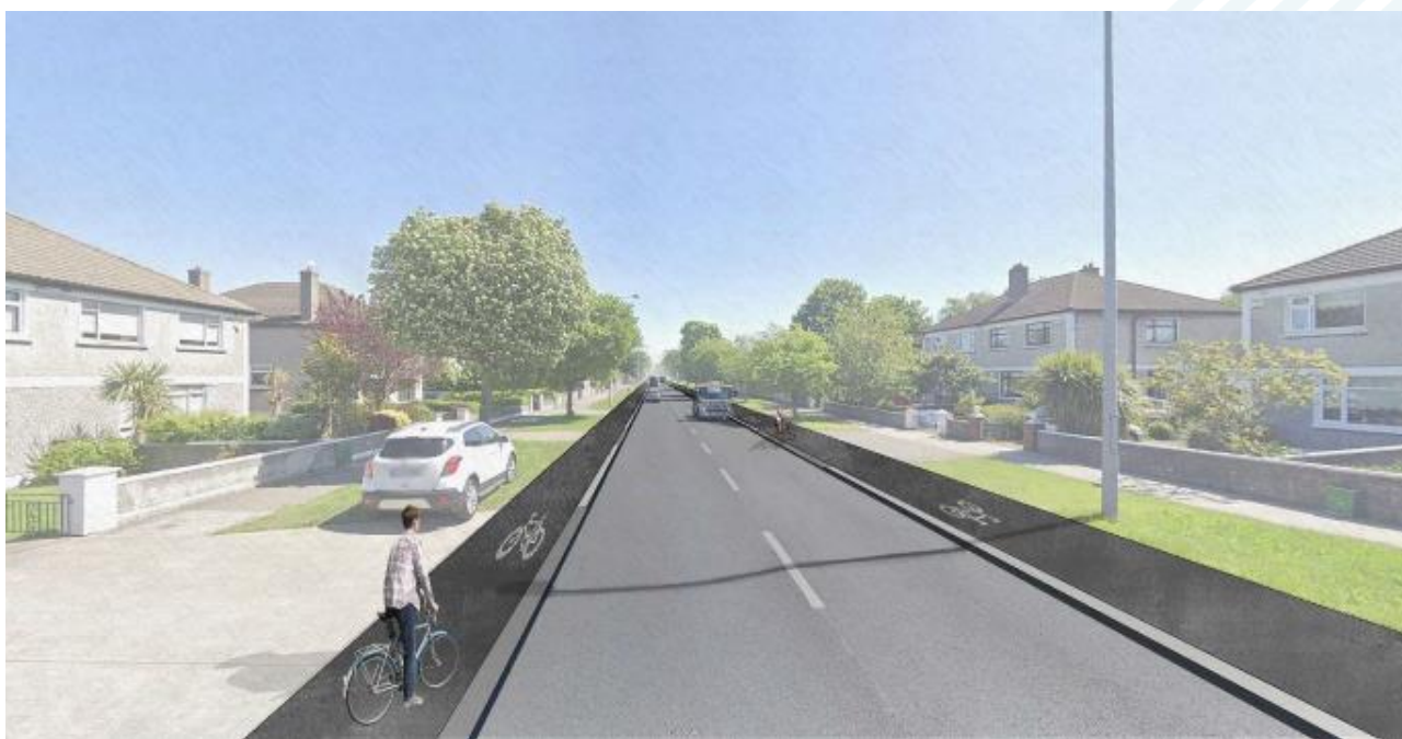
Figure 2-3: Proposed permanent layout of Templeville road with cycle lanes on either side (Overlaid on Google Street View, 2021).
