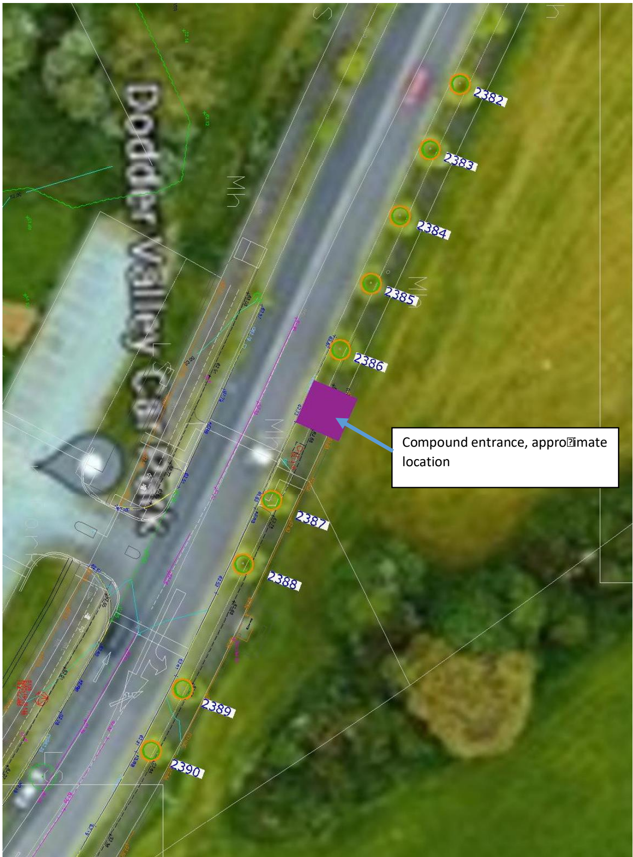
Figure 22 Location of street trees either side of contractor's compound entrance
