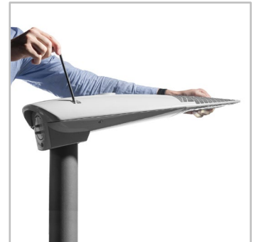
Universal fixation for side-entry or post-top mounting with adjustable inclination in steps of 2.5^\circ .
