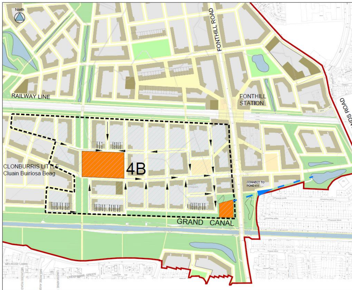
Figure 5-7: Strategic Drainage Approach to Sub-catchment 4b
