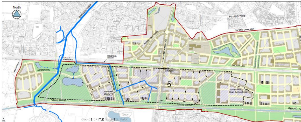
Figure 5-9: Strategic Drainage Approach to Sub-catchment 5
