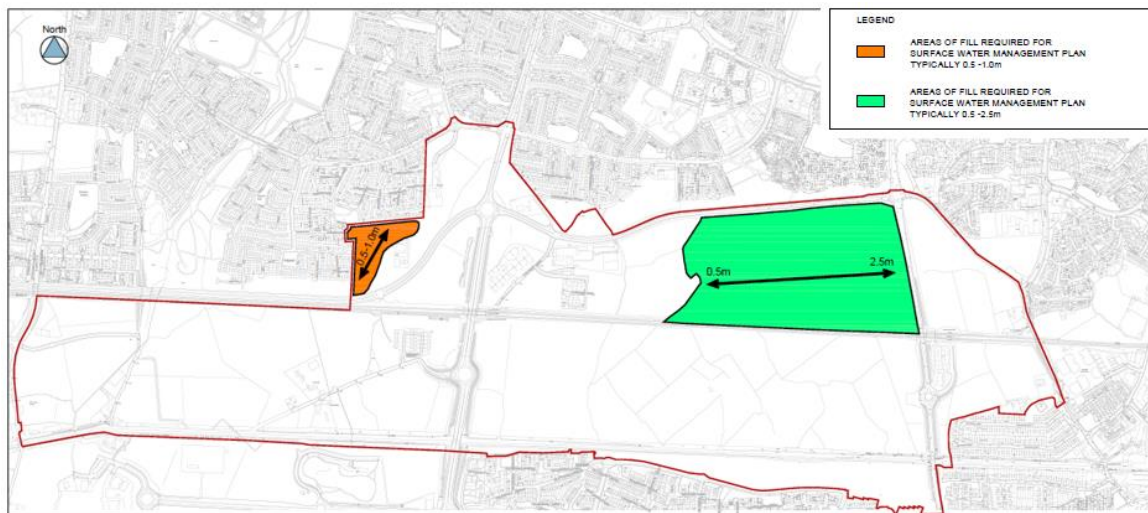
Figure 4-2: Required Fill Depths
