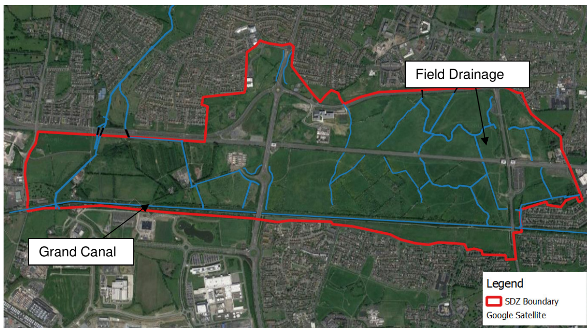
Figure 2-3: Field Drainage in SDZ
