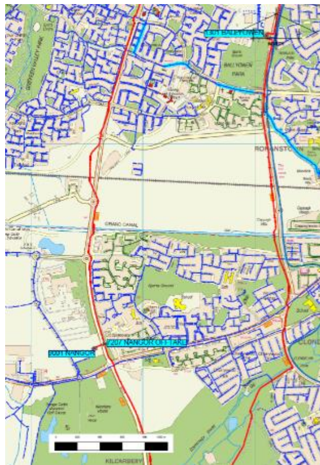
Figure 27: Gas infrastructure map showing high pressure gas transmission pipes (shown in red) in the vicinity of the SDZ [Source: Gas Networks Ireland via SDCC]
