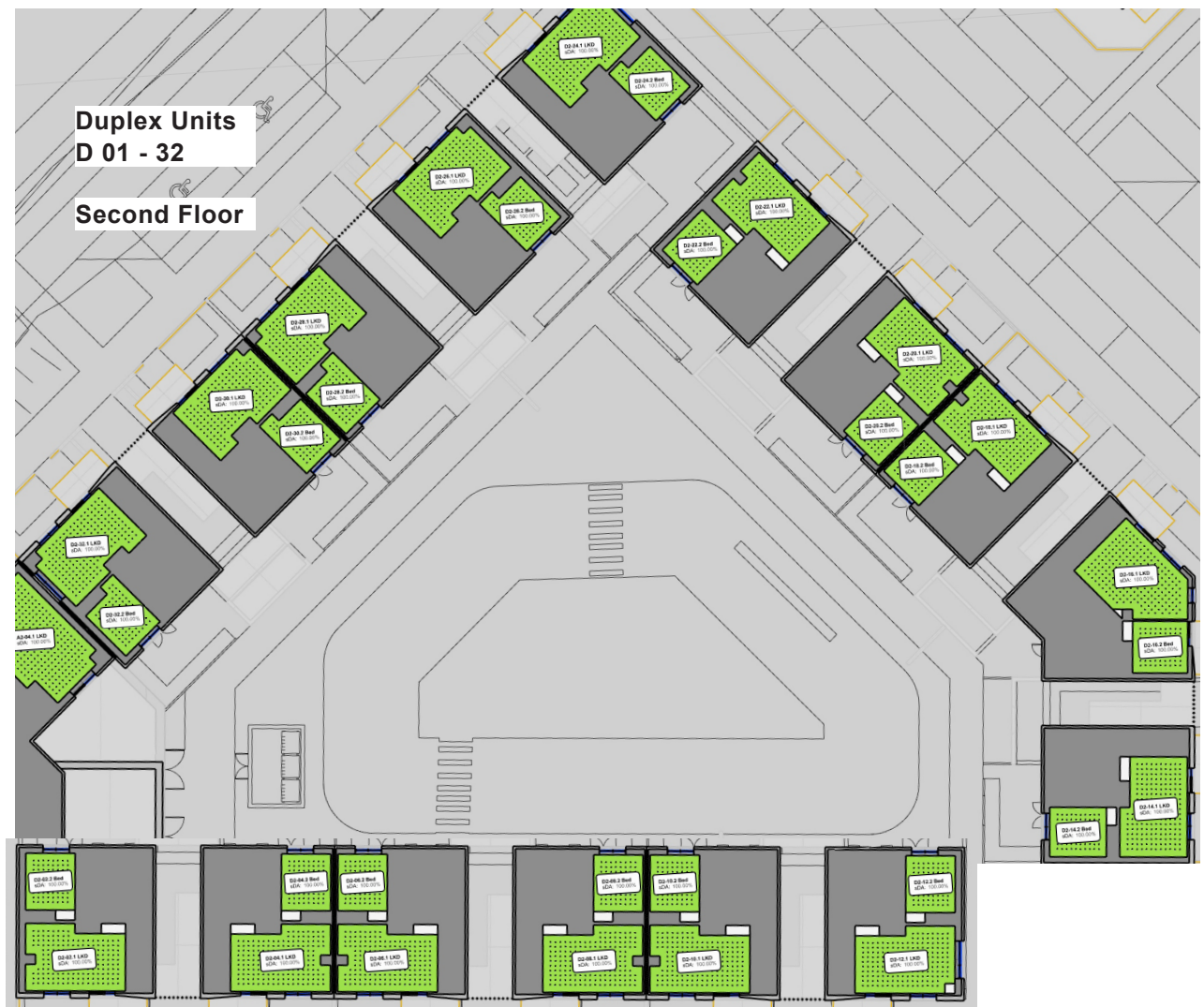
Figure 24: Floor plans indicating Daylight Provision to BS EN17037:2021+A1 Table NA.1
