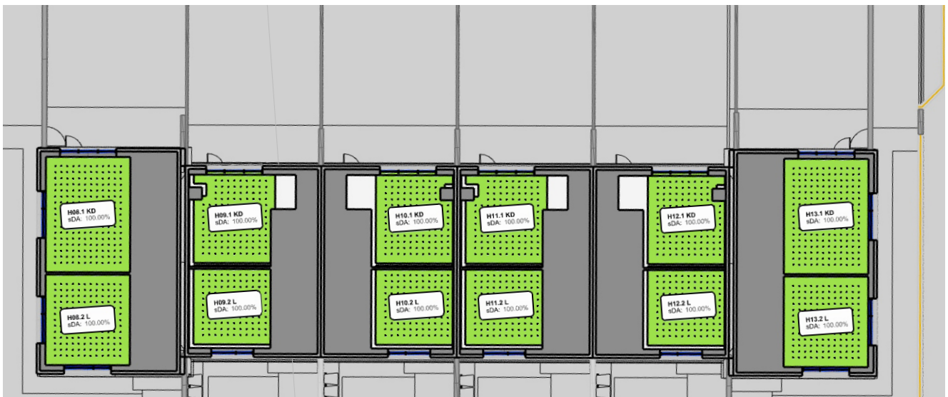
Figure 27: Floor plans indicating Daylight Provision to BS EN17037:2021+A1 Table NA.1
