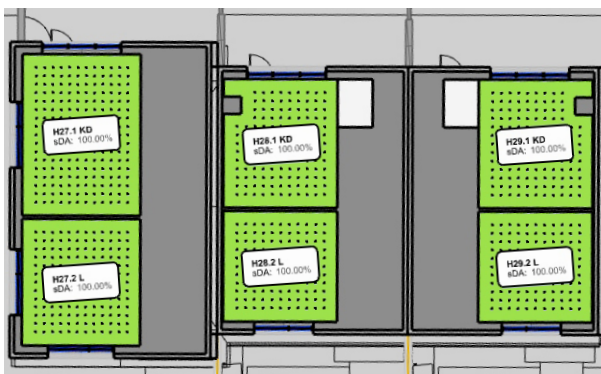
Figure 29: Floor plans indicating Daylight Provision to BS EN17037:2021+A1 Table NA.1
