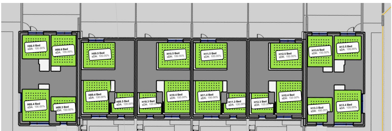
Figure 28: Floor plans indicating Daylight Provision to BS EN17037:2021+A1 Table NA.1
