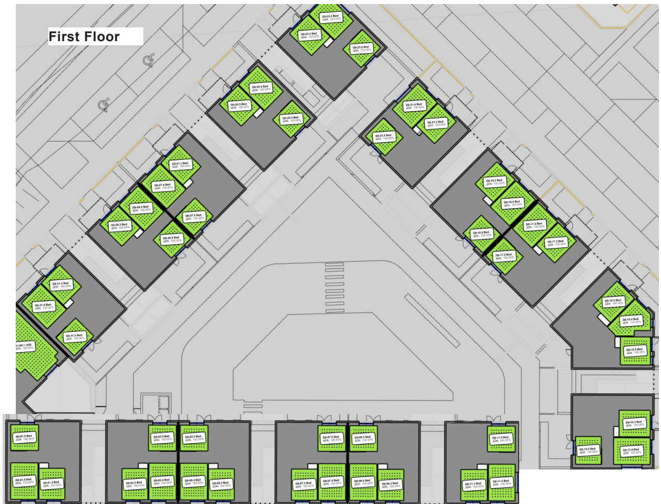
Figure 23: Floor plans indicating Daylight Provision to BS EN17037:2021+A1 Table NA.1
