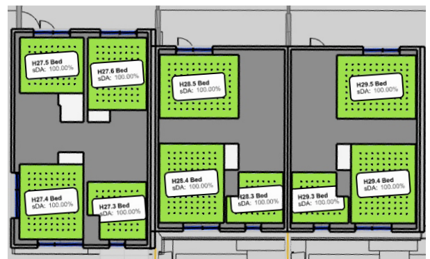
Figure 29: Floor plans indicating Daylight Provision to BS EN17037:2021+A1 Table NA.1
