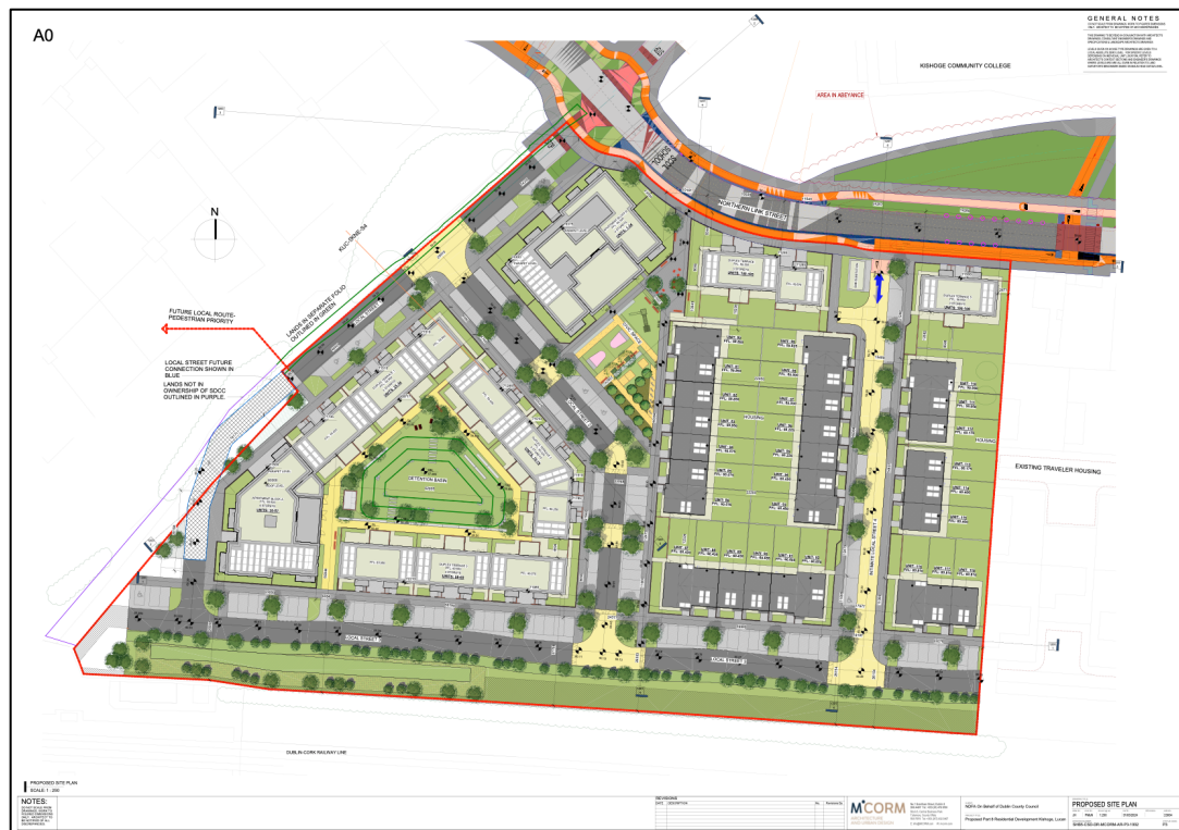
Figure 2: Extract from drawing “SHB5-CSD-DR-MCORM-AR-P3-1002 Plan” showing the proposed roof layouts with the location of the proposed PV panels.
