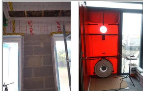
*Figure 3: Air tightness testing examples*
