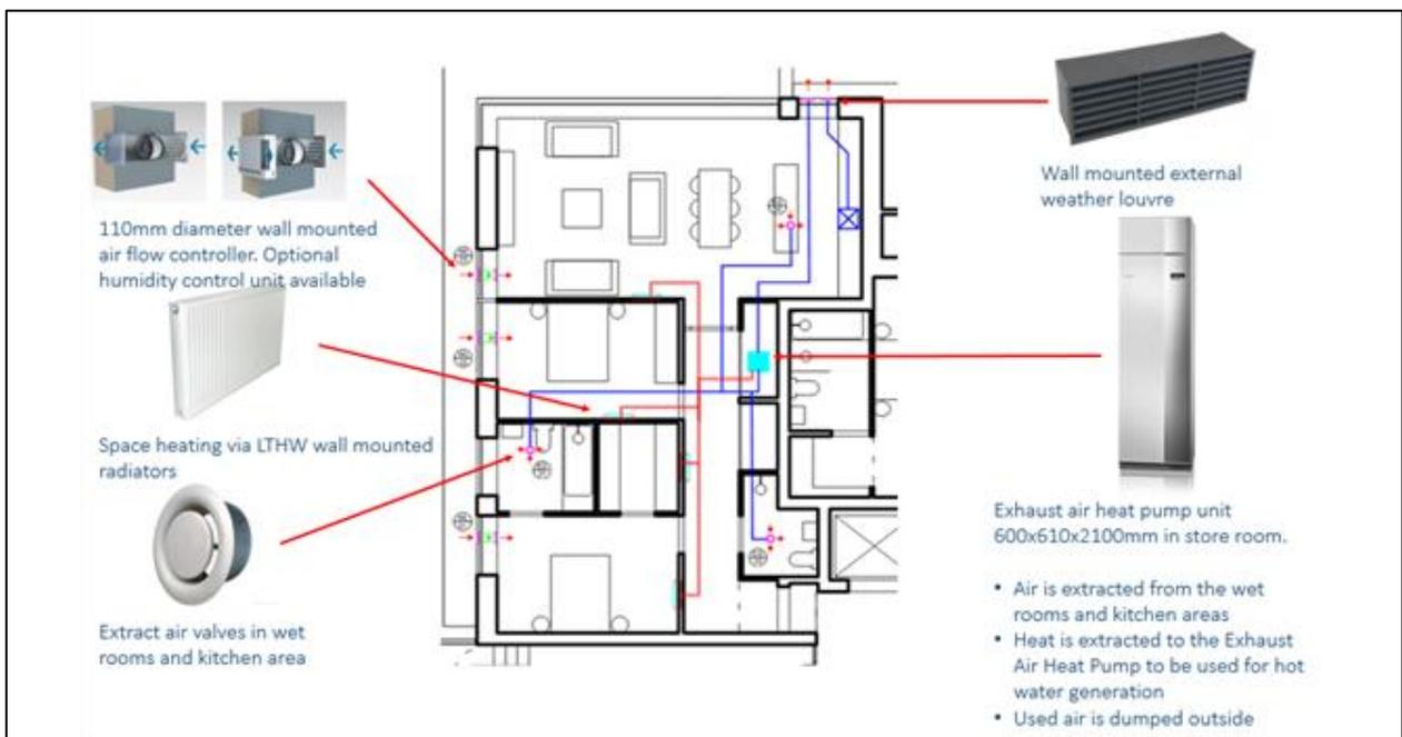
*Figure 7: Example Diagram of Typical Exhaust Air Heat Pump Layout*
