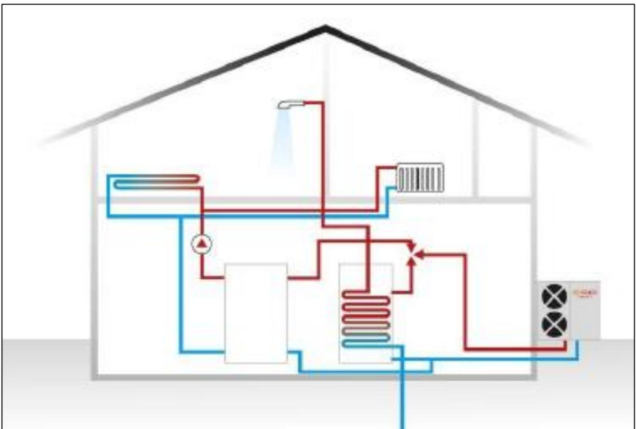
*Figure 5: Air-Source Heat Pump Diagram*
