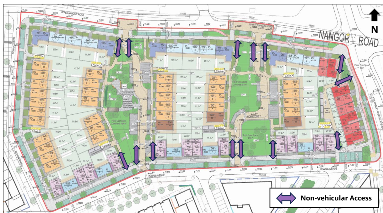
Figure 4-3: Non-vehicular Access Locations (Source: Burke-Kennedy Doyle Architects)
