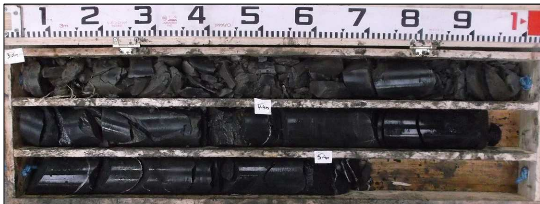
Photo 1 – Core recovery at RC05 (3.0 – 5.4 m BGL) showing highly fractured upper bedrock from 3.0-3.5m
