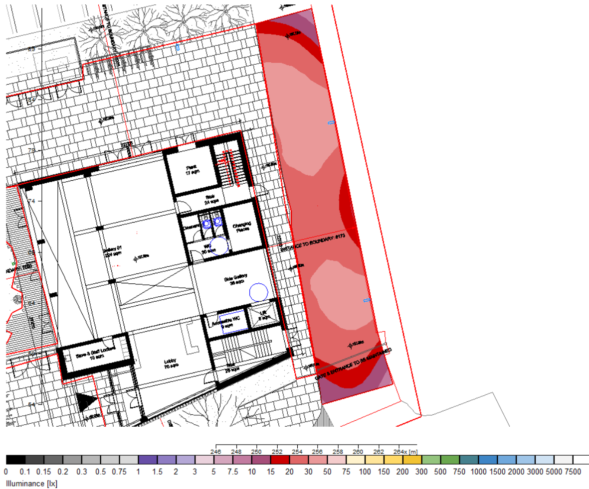
Figure 5.1.1 - Illumination Levels at the Entrance Road
