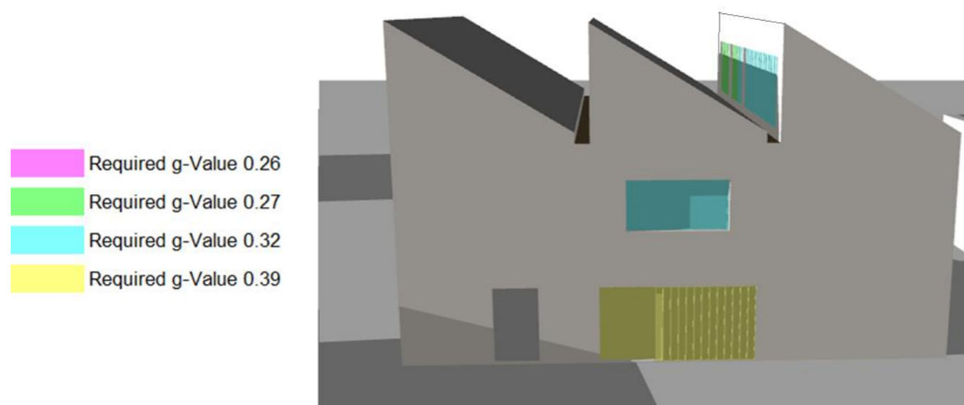
Fig 8.1.1 – North Elevation – Required Solar Performance for Glazing
