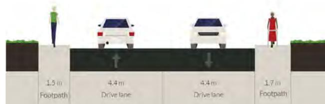
**Figure 6.11 - Route 3, Cross Section A-A Existing**
