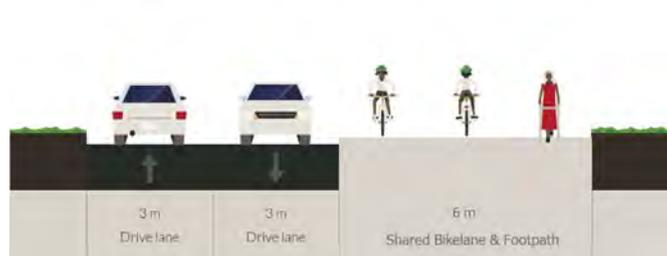
**Figure 6.9 - Route 2B, Cross Section A-A Proposed**
