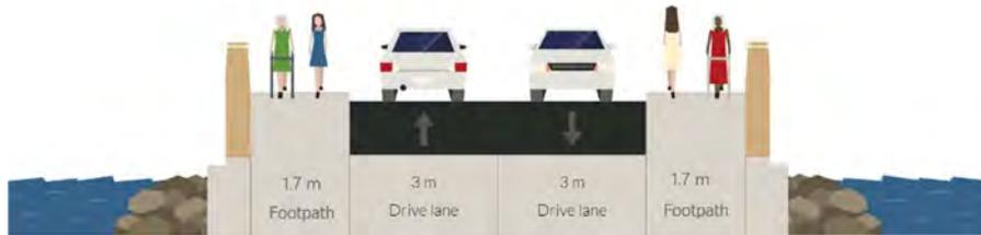
**Figure 8.14 - Route 11, Cross Section A-A Existing**
