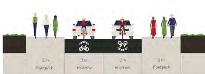
Figure 6.23 - Route 4-1A & 4-2A Cross Section A-A Proposed
