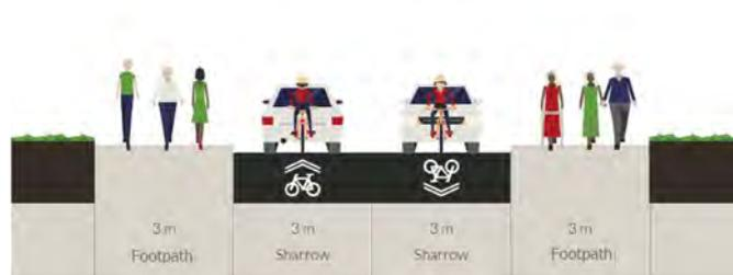
**Figure 6.12 - Route 3A, Cross Section A-A Proposed**
