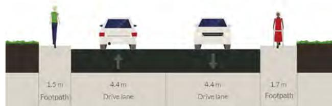
**Figure 6.36 - Route 5, Cross Section A-A Existing**
