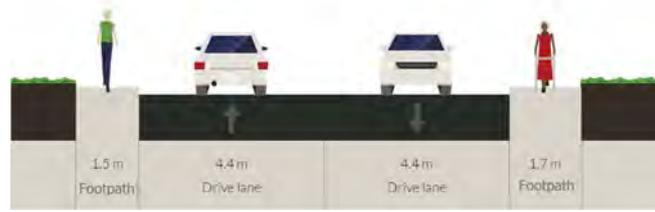
Figure 6.22 - Route 4, Cross Section A-A Existing
