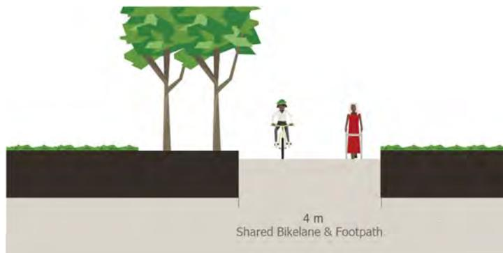
**Figure 5.4 - Route 1A, Cross Section A-A Proposed**
