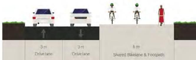
**Figure 6.35 - Route 5B Cross Section A-A Proposed**
