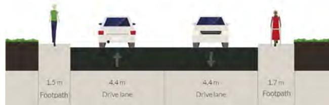
**Figure 6.34 - Route 5, Cross Section A-A Existing**
