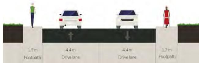
**Figure 6.3 - Route 2, Cross Section A-A Existing**
