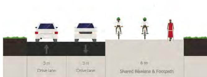
Figure 6.17 - Route 3B, Cross Section A-A Proposed
