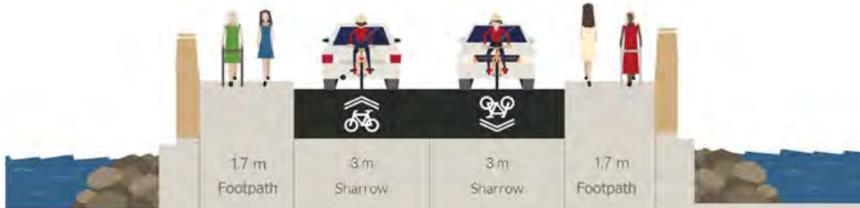
**Figure 8.22 - Route 13 A & 13 B, Cross Section A-A Proposed**
