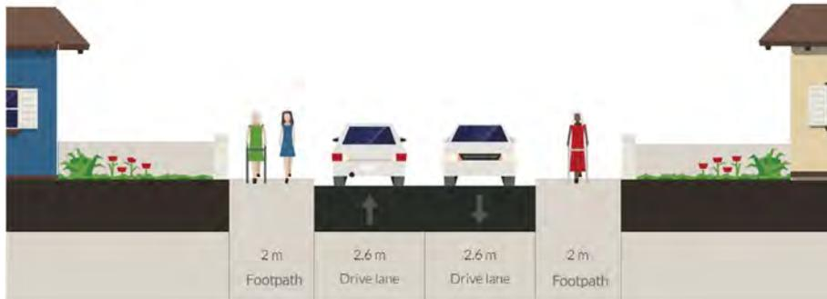
Figure 6.24 - Route 4, Cross Section B-B Existing
