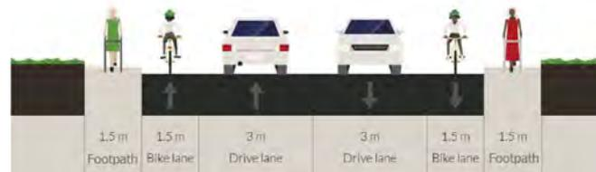
**Figure 6.37 - Route 5C Cross Section A-A Proposed**
