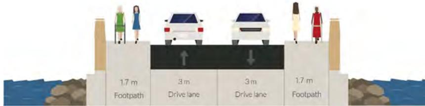
**Figure 8.21 - Route 13, Cross Section A-A Existing**
