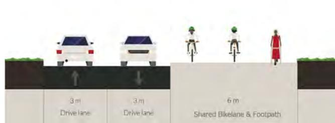
**Figure 6.27 - Route 4-1B & 4-2B Cross Section A-A Proposed**
