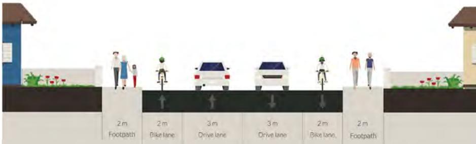
Figure 6.47 - Route 6C, Cross Section A-A Proposed
