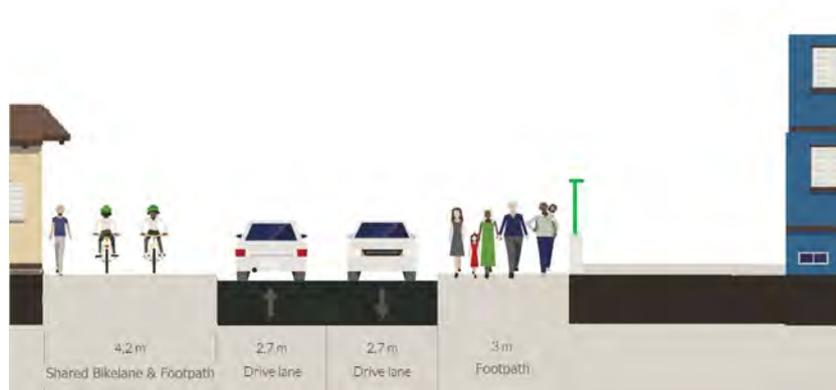
**Figure 6.52 - Route 7A, 7B & 7C, Cross Section B-B Proposed**
