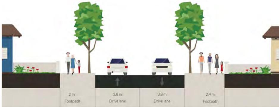
Figure 6.64 - Route 8, Cross Section A-A Existing
