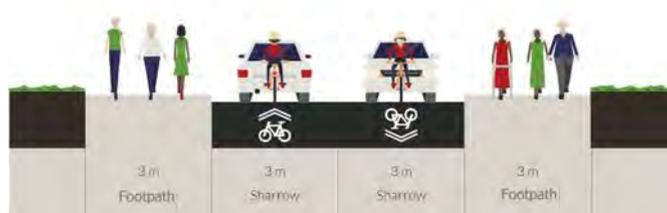
**Figure 6.4 - Route 2, Cross Section A-A Proposed**
