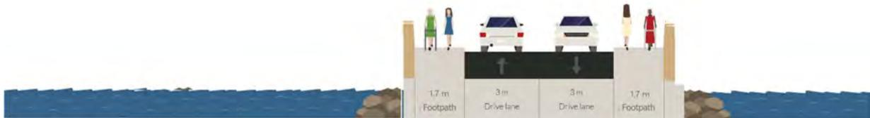
Figure 8.18 - Route 12, Cross Section A-A Existing
