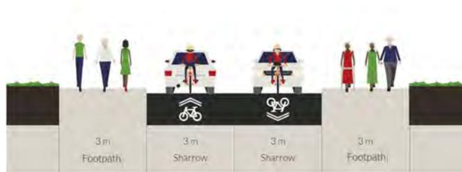
**Figure 6.31 - Route 5A Cross Section A-A Proposed**
