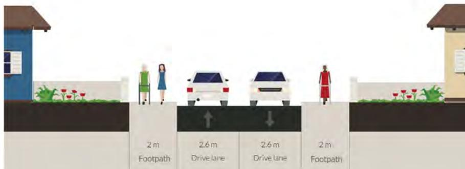
Figure 6.42 - Route 6, Cross Section B-B Existing
