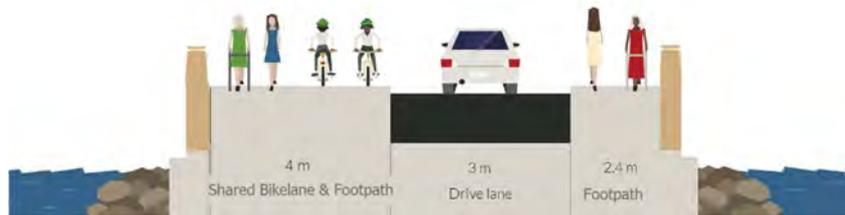
**Figure 8.24 - Route 13 C, Cross Section A-A Proposed**
