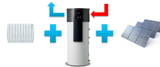
Figure 2: Electrical Space Heating, Domestic Hot Water Air to Water Heat Pump and Photovoltaics
