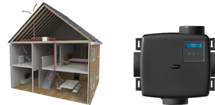
Figure 7: Typical CME layout in a dwelling and typical CME extract unit
