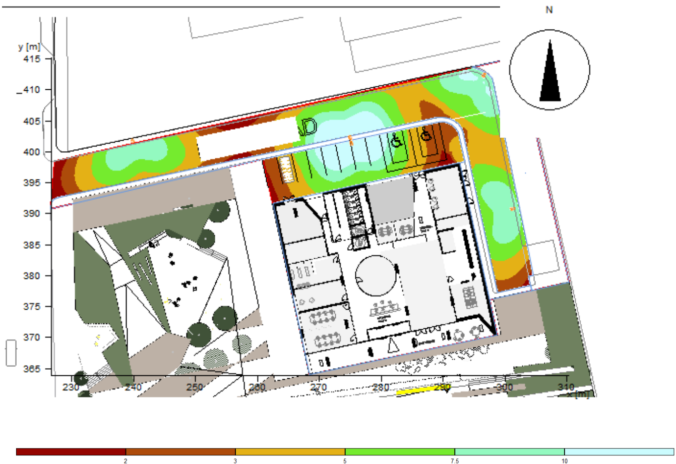
Figure 5.1.1 - Illumination Levels at the Entrance Road
