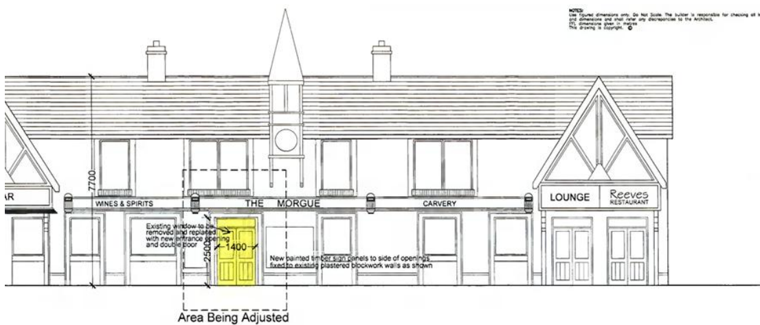
Figure 3: SD20A/0276 Proposed Elevations (Source: SDCC)
