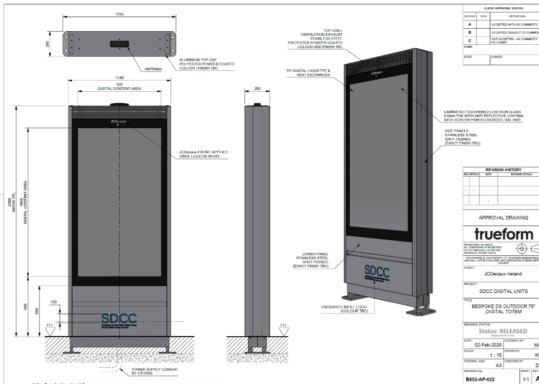
Figure 5 Technical detail of proposed Digipanel
