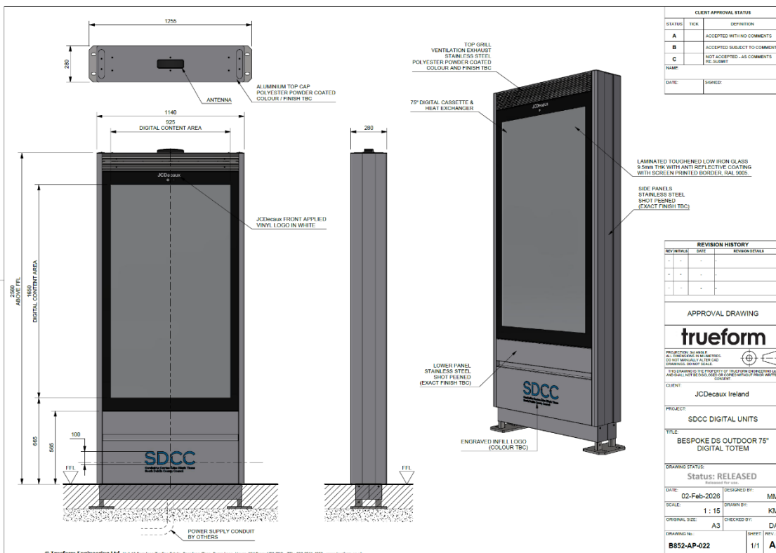
Figure 4 Technical detail of proposed Digipanel
