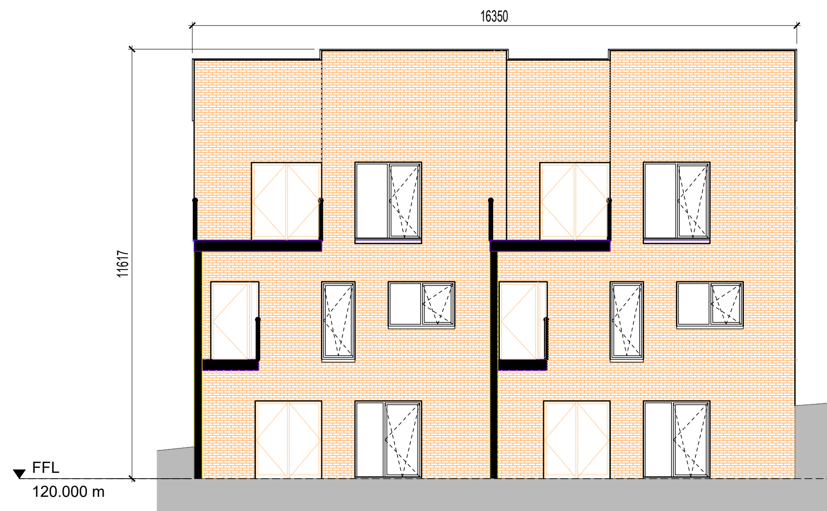
2 BUILDING 1 REAR ELEVATION 1:100 (A1)
