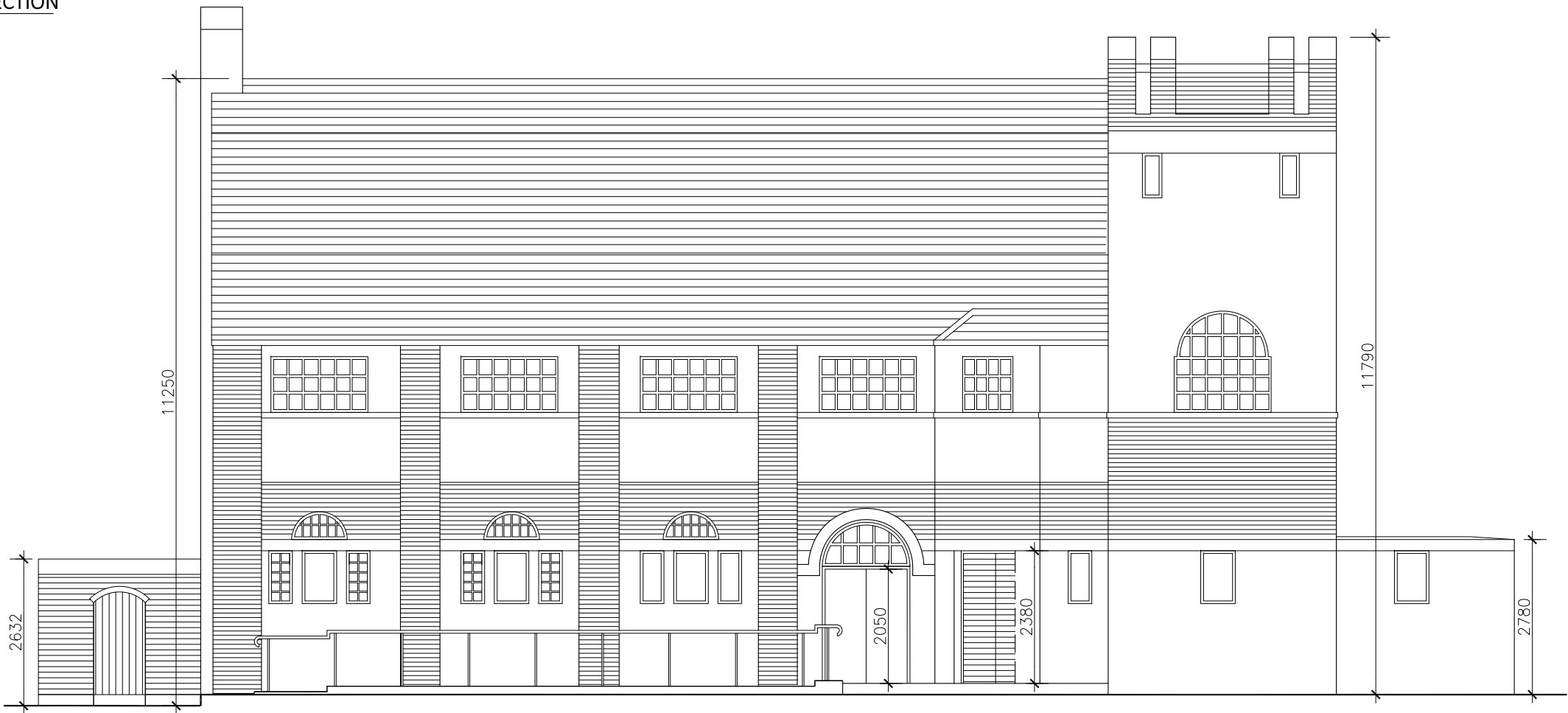
EXISTING FRONT ELEVATION Scale 1:100
