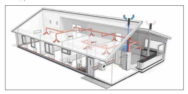
Figure 6: Example Diagram of Typical Exhaust Air Heat Pump Layout
