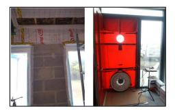
Figure 3: Air tightness testing examples
