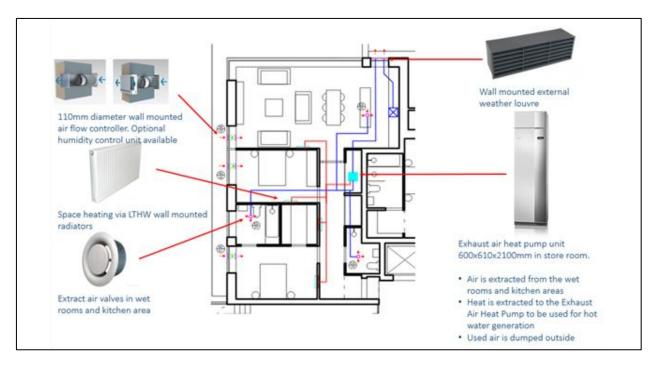
Figure 7: Example Diagram of Typical Exhaust Air Heat Pump Layout
