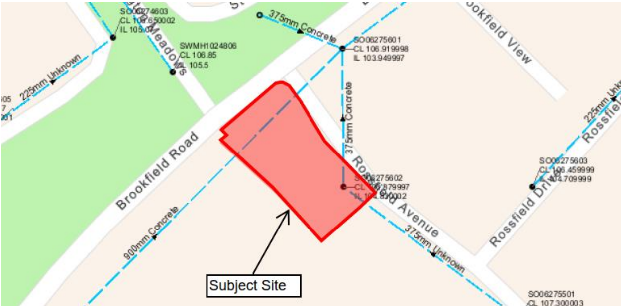
Figure 4-1: Existing Surface Water Drainage in the Vicinity of the Site – as per GIS records
