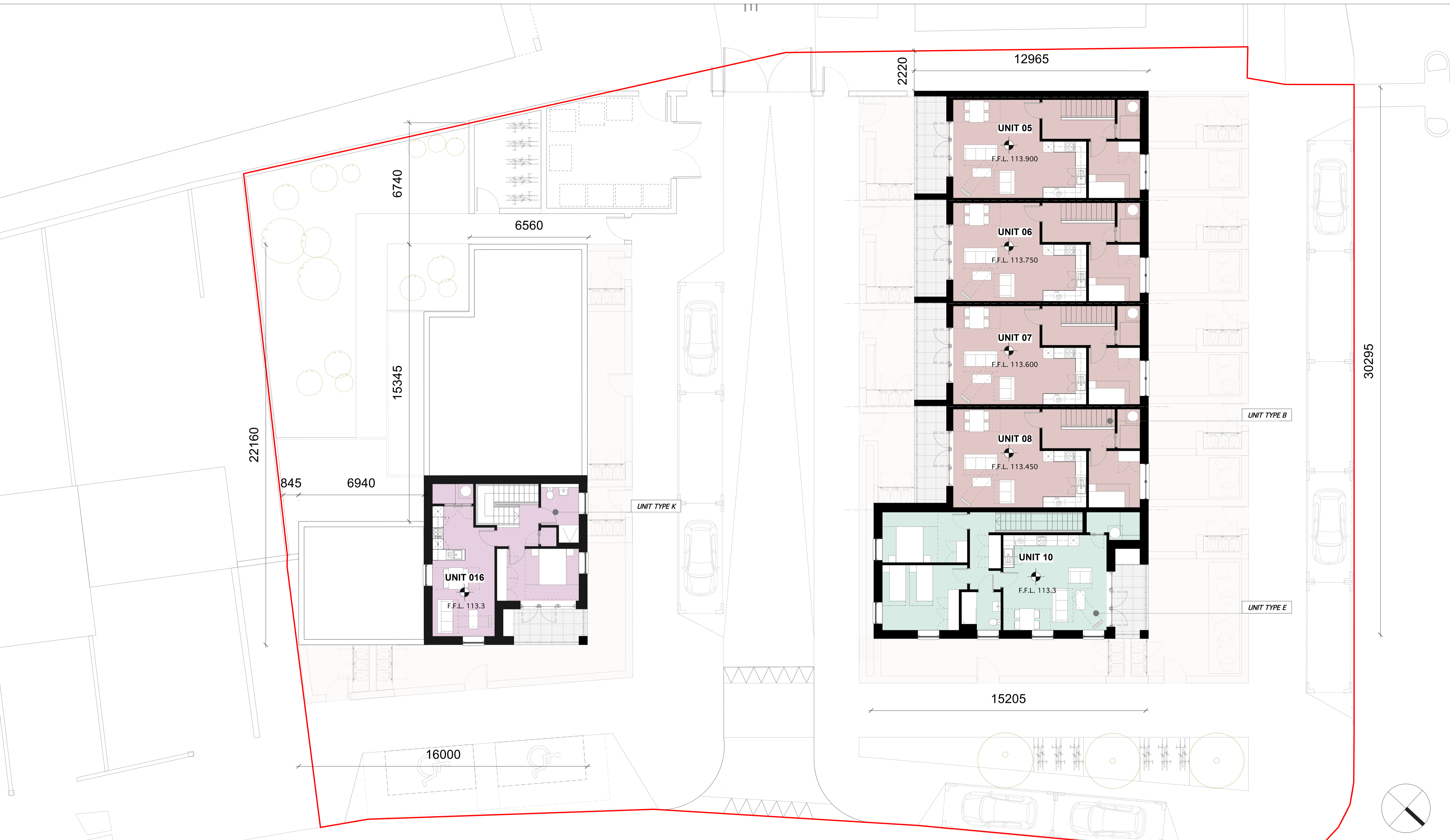
1 PA-003 PROPOSED SECOND FLOOR PLAN 1:100 @A1 / 1:200 @A3
