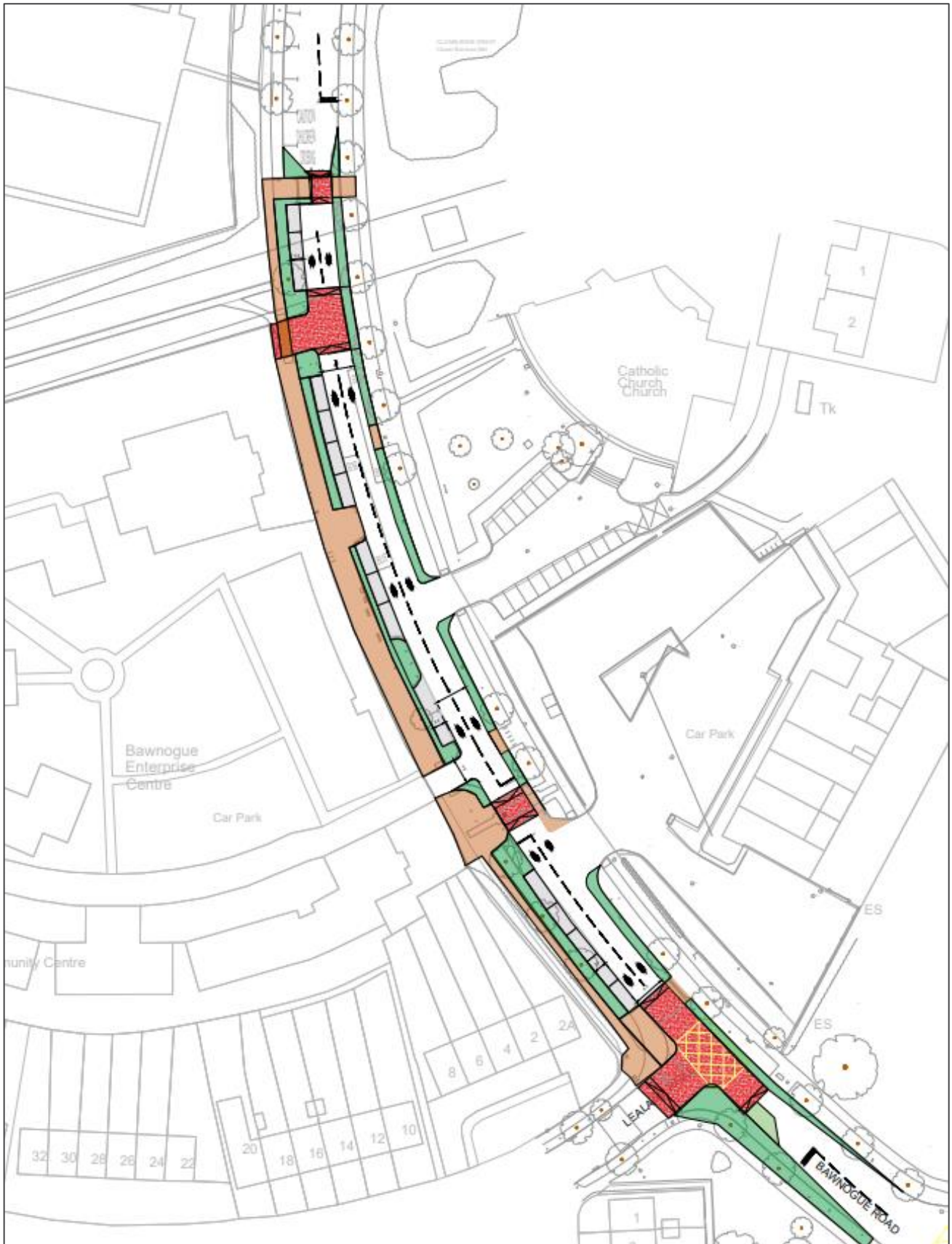
Figure 1.4. Retention of on-street parking. Reduction of carriageway width to 6m. On-street cycle roundel lining to highlight presence of cyclist in carriageway.
